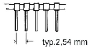
Ø hole in PCB typ. 1,0 mm
