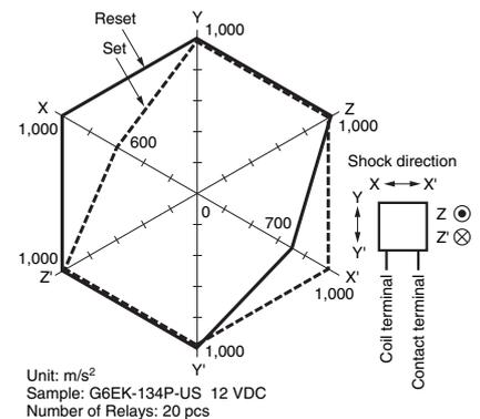
Test Conditions: Shock is applied in ±X, ±Y, and ±Z directions three times each with and without energizing the Relays to check the number of contact malfunction.
