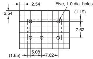
**Terminal Arrangement/ Internal Connections**
