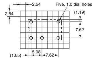
**Terminal Arrangement/ Internal Connections**
