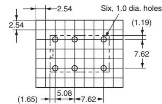
**Terminal Arrangement/ Internal Connections**
