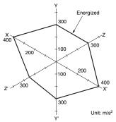
Sample: G6B-1114P-US Number of Relays: 12 pcs Test Conditions: Shock is applied in  $\pm X$ ,  $\pm Y$ , and ±Z directions three times each with without energizing the Relays Shock direction to check the number of malfunctions. z 💿 Requirement: None z¹⊗ malfuction 100 m/s<sup>2</sup>
