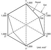
Sample: G6BK-1114P-US Number of Relays: 12 pcs Test Conditions: The value at which malfunction occurred was measured after Shock direction applying shock to the test piece 3 times each in 6 directions along 3 axes.  $Z' \otimes$ Standard value: (Coil) 300 m/s<sup>2</sup>
