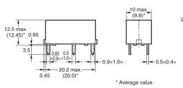
Dimensions in pointed brackets < > are for the G6B-P(-FD)-US-P6B Socket Relay.
