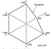
Sample: G6B-1174P-US G6B-1174P-FD-US Test Conditions: Shock is applied in ±X, ±Y, and ±Z directions three times each with without Shock direction energizing the Relays to check the number of malfunctions. Requirement: None malfuction 100 m/s2 (Coil)
