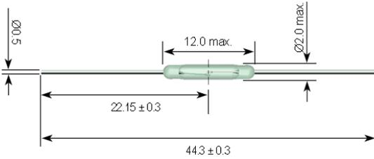
tolerances according to DIN ISO 2768 m
