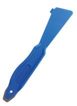
The Multi-Opener can be used for the gentle opening of sensitive equipment and for working on clipped housings. The Opener is produced entirely in Germany and is made of glass-fibre reinforced polyamide as well as a dissipative ESD material, which protects against electrostatic discharges.
