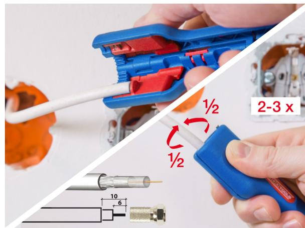
The Coax-Stripper No. 1 F Plus enables a quick and easy stripping of coaxial cables in just one single step. The two opposite pairs of knives allow a fast and space-saving stripping process with a few gentle rotation movements. The preadjusted sheath opening is suitable for common F-connectors (6 / 4 mm). If needed, the knife inserts can be exchanged in order to be suitable for different sheath openings, e.g. for compression connectors (6,5 / 6,5 mm).
