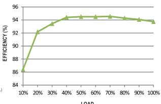
The curve above is measured at 230VAC.
