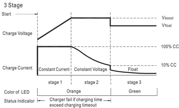
☉ Suitable for lead-acid batteries (flooded, Gel and AGM) and Li-ion batteries (lithium iron and lithium manganese).
