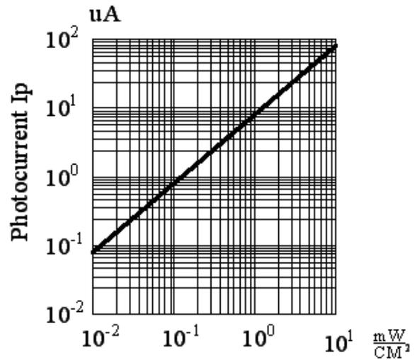
Fig6 PHOTOCURRENT VS IRRADIANCE  $\lambda = 940nm$
