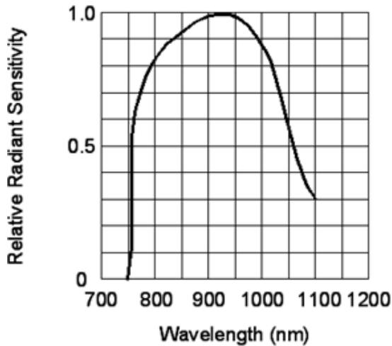
FIG.5 SPECTRAL SENSITIVITY
