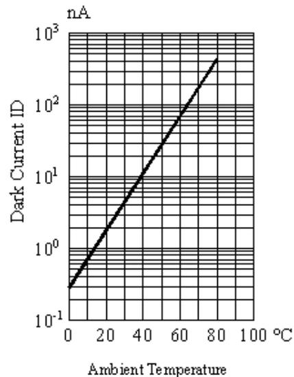
Fig.4 DARK CURRENT AMBIENT TEMPERATURE
