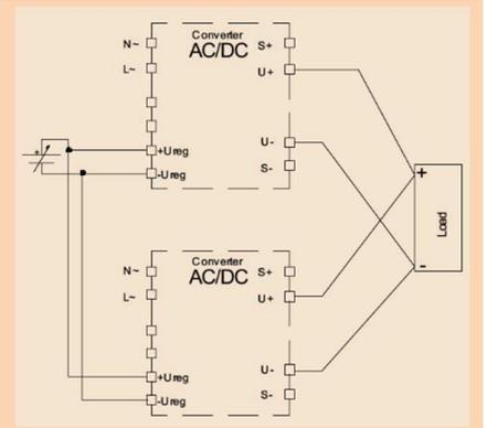
The HSEUREG models have no internal O-ring diode, to operate the devices N+1 redundant.
