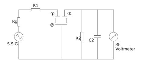
$R1=280\Omega\pm5\%, R2=330\Omega\pm5\%, Rg=50\Omega$  :Input C2=10 Pf (Including stray capacitance and capacitance of RF Voltmeter) :Output S.S.G:Output Voltmeter
