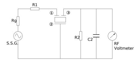
$\begin{array}{ll} R1+Rg=R2=330\Omega\pm5\%, Rg=50\Omega & :Input \\ C2=10 \ PF \ (Including \ stray \ capacitance \\ and \ capacitance \ of \ RF \ Voltmeter) & :Output \\ S.S.G:Output \ Voltmeter & :Output \end{array}$
