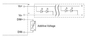
"DO NOT connect "DIM- to -V"
