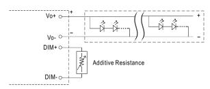
"DO NOT connect "DIM- to -V"
