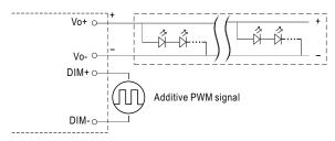
"DO NOT connect "DIM- to -V"
