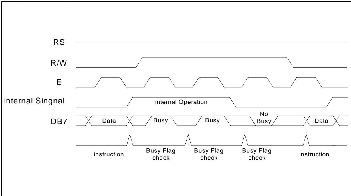
Example of 8-bit bus mode timing diagram
