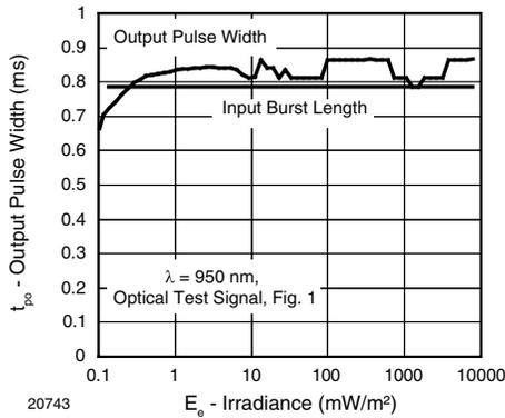
Figure 2. Pulse Length and Sensitivity in Dark Ambient
