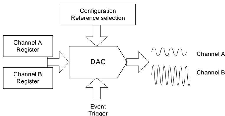
The DAC has one continuous output with high drive capabilities for both resistive and capacitive loads. It is also possible to split the continuous time channel into two Sample and Hold (S/H) channels, each with separate data conversion registers.
