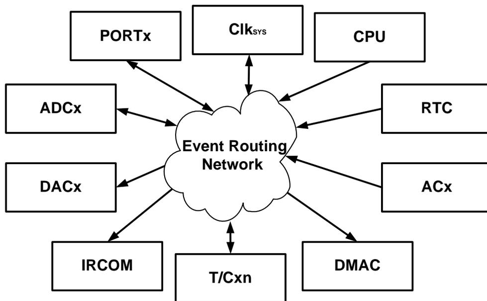
The Event Routing Network can directly connect together ADCs, DACs, Analog Comparators (ACx), I/O ports (PORTx), the Real-time Counter (RTC), Timer/Counters (T/C) and the IR Communication Module (IRCOM). Events can also be generated from software (CPU).
