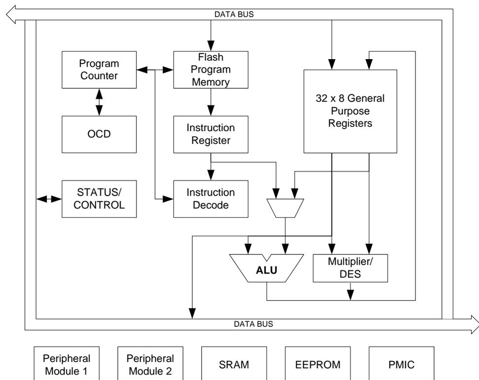
The AVR uses a Harvard architecture - with separate memories and buses for program and data. Instructions in the program memory are executed with a single level pipeline. While one instruction is being executed, the next instruction is pre-fetched from the program memory. This
