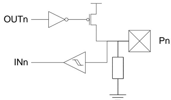
Figure 14-6. I/O configuration - Wired-AND with optional pull-up
