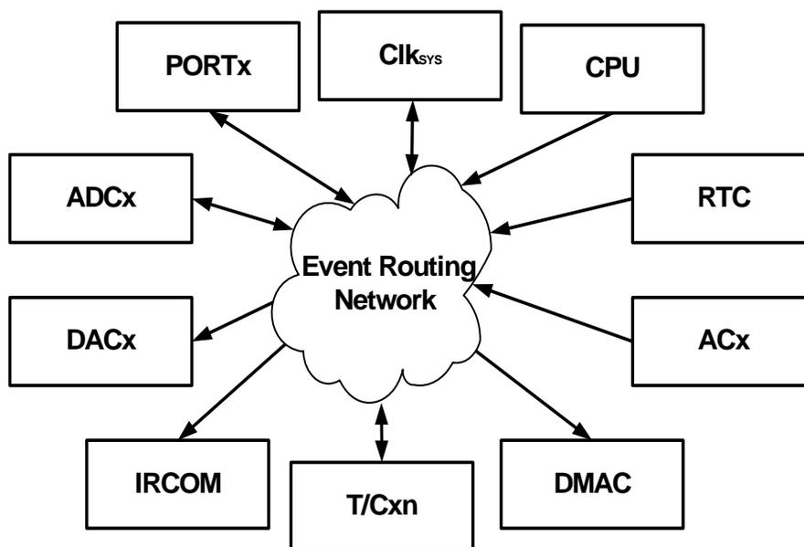
The Event Routing Network can directly connect together ADCs, DACs, Analog Comparators (ACx), I/O ports (PORTx), the Real-time Counter (RTC), Timer/Counters (T/C) and the IR Communication Module (IRCOM). Events can also be generated from software (CPU).
