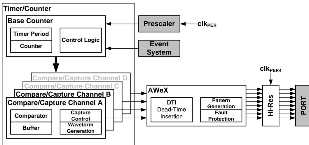
The Hi-Resolution Extension can be enabled to increase the waveform generation resolution by 2 bits (4x). This is available for all Timer/Counters. See ["Hi-Res - High Resolution Extension"](#) on page 33 for more details.
