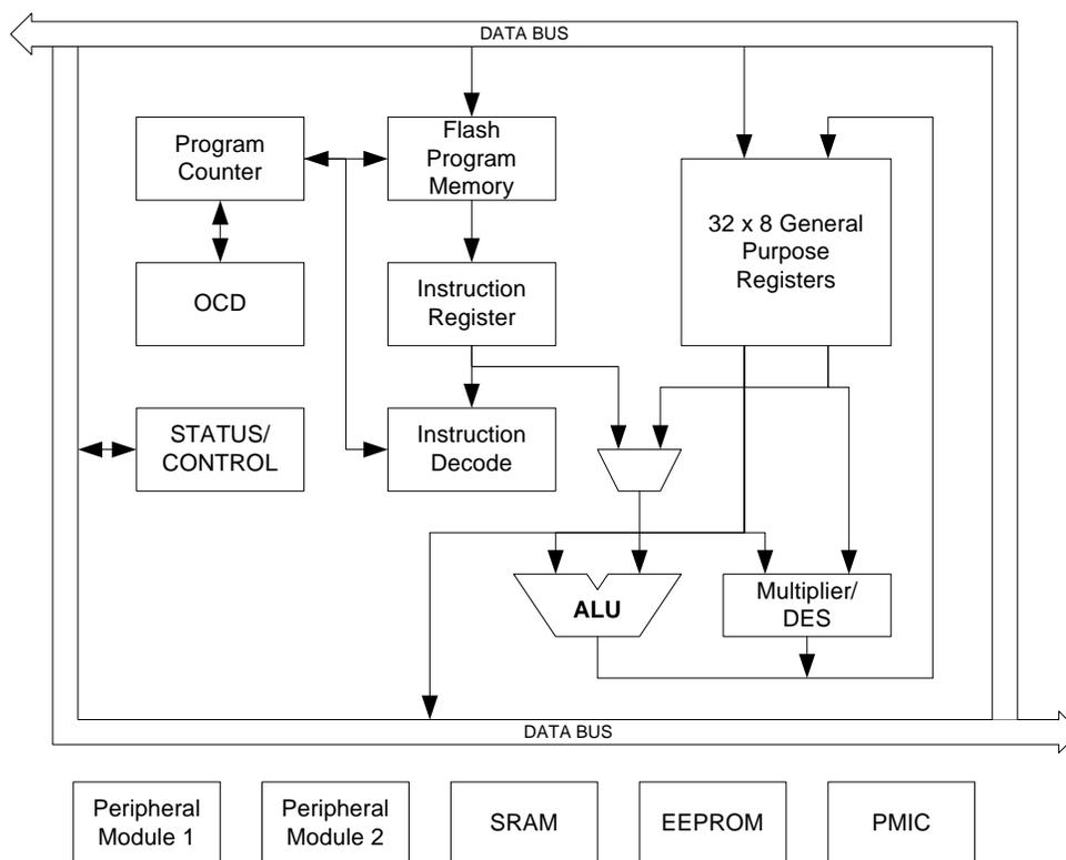
The AVR uses a Harvard architecture - with separate memories and buses for program and data. Instructions in the program memory are executed with a single level pipeline. While one instruction is being executed, the next instruction is pre-fetched from the program memory.
