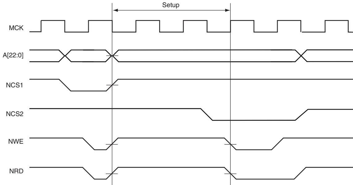
**Figure 18-24.** First Access with Data Float Wait States (TDF = 2) and Second Access with Setup (NRDSETUP = 1)
