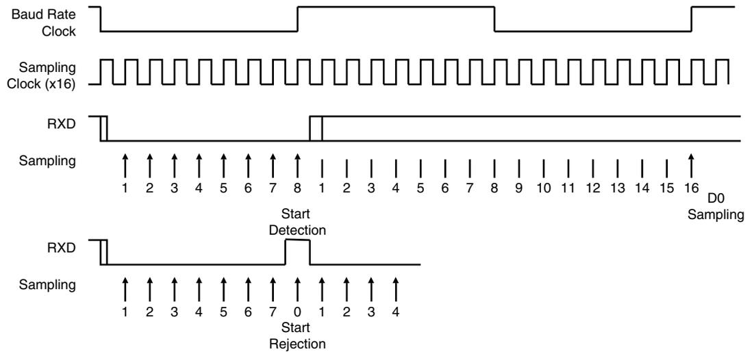
**Figure 30-8.** Asynchronous Character Reception
