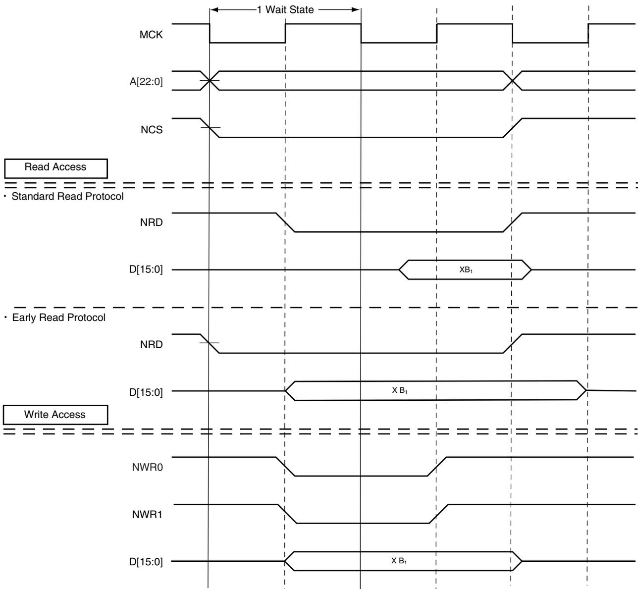
**Figure 18-44. 0 Wait State, 16-bit Bus Width, Byte Transfer**
