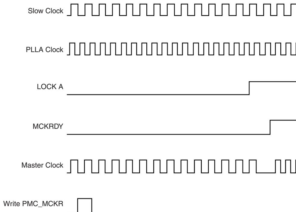
**Figure 23-10. Switch Master Clock from Main Clock to Slow Clock**
