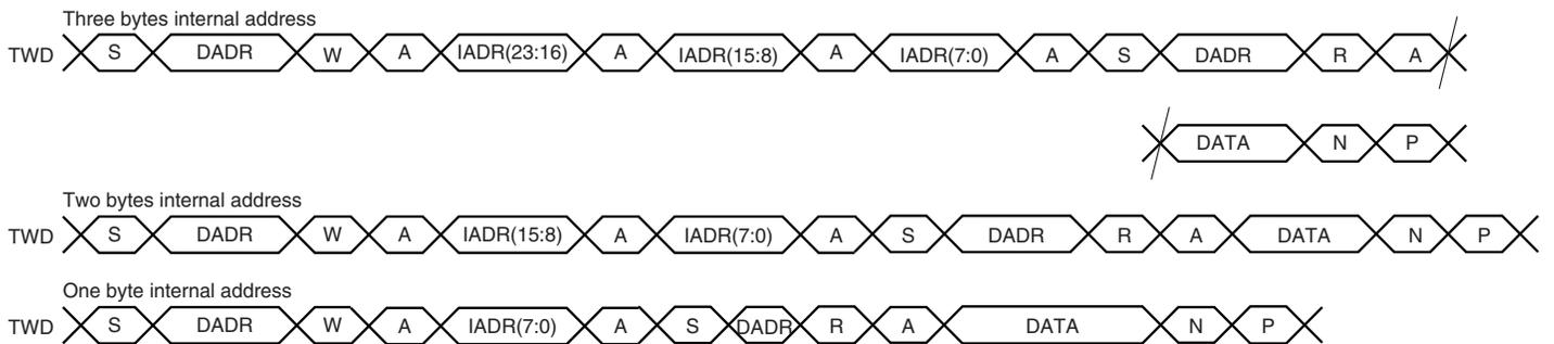
**Figure 29-8. Master Read with One Byte Internal Address and Multiple Data Bytes**
