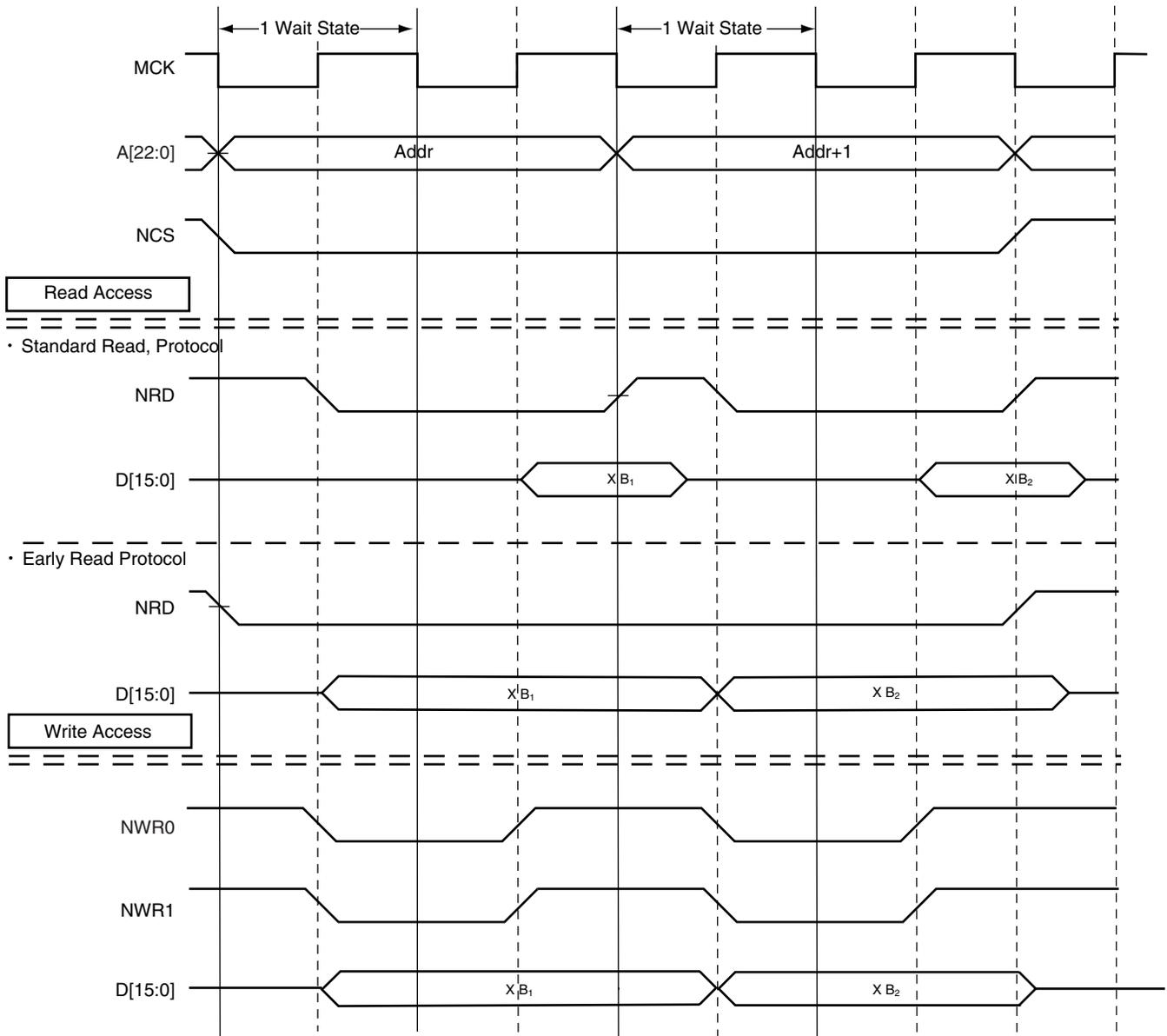
Figure 18-43. 1 Wait State, 8-bit Bus Width, Byte Transfer
