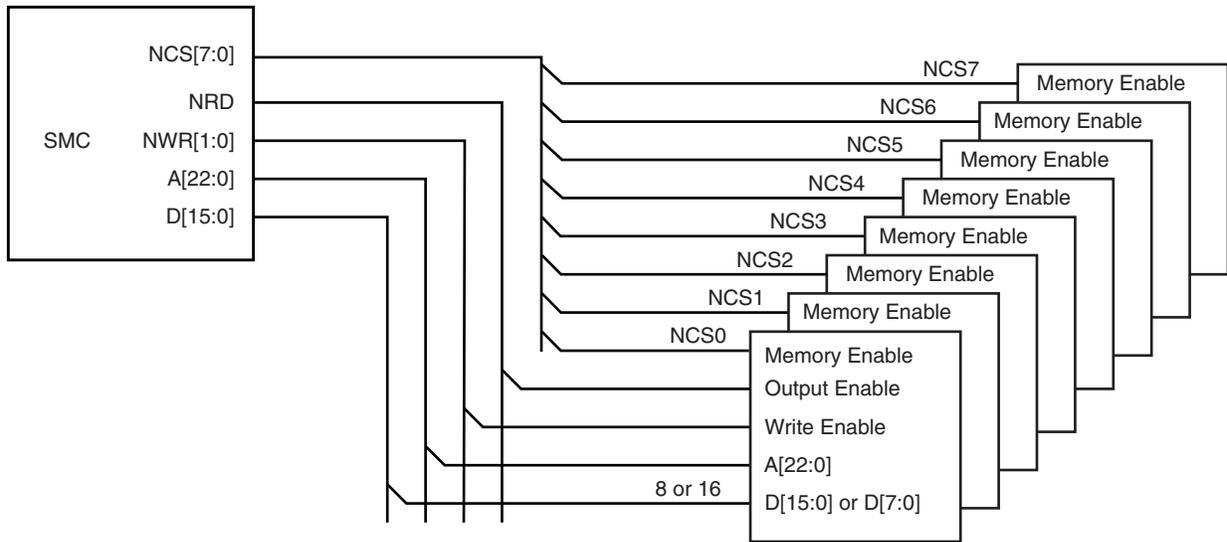
Note: 1. The maximum address space per device is 8 Mbytes.
