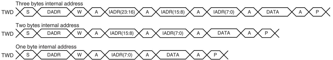
**Figure 29-6. Master Write with One Byte Internal Address and Multiple Data Bytes**
