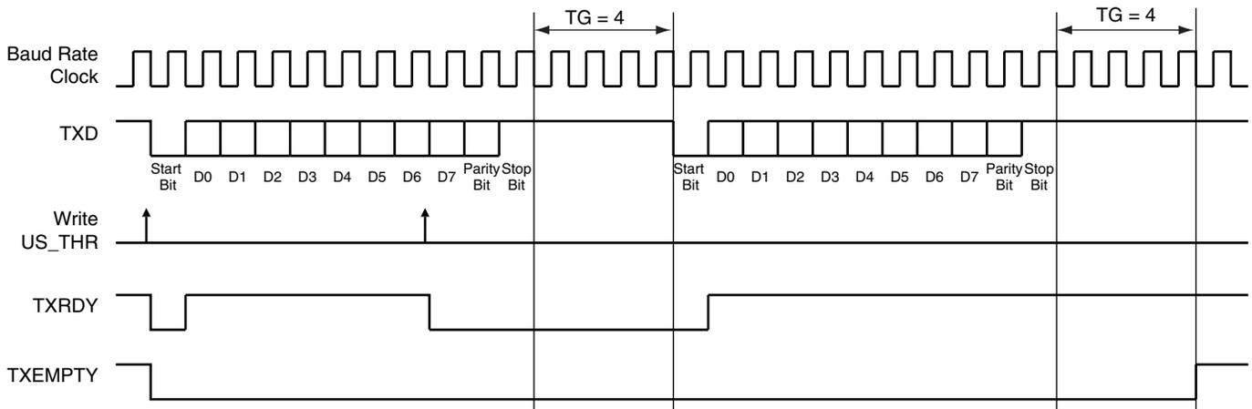
Table 30-7 indicates the maximum length of a timeguard period that the transmitter can handle in relation to the function of the Baud Rate.
