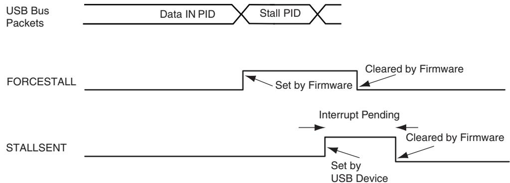
**Figure 34-15.** Stall Handshake (Data OUT Transfer)
