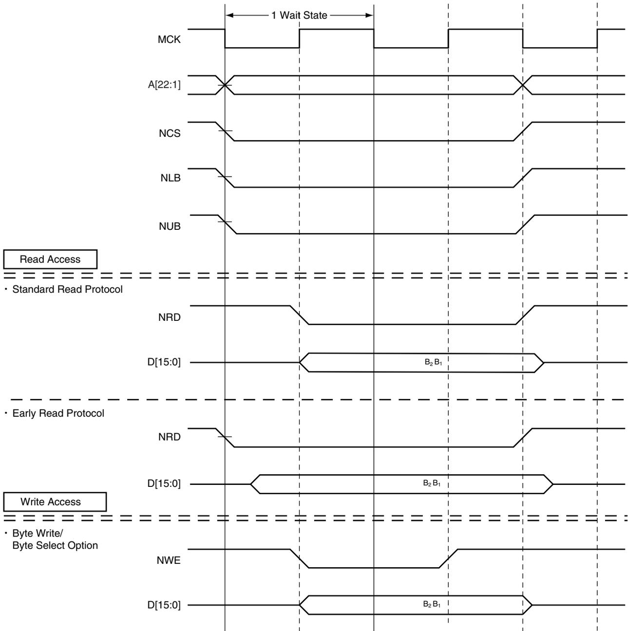
Figure 18-41. 0 Wait State, 8-bit Bus Width, Word Transfer
