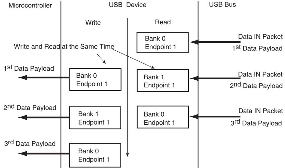
When using a ping-pong endpoint, the following procedures are required to perform Data OUT transactions:
