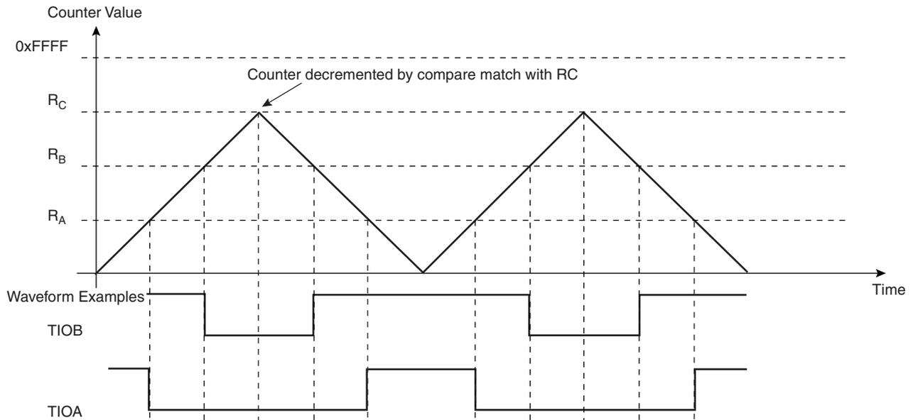
**Figure 32-13. WAVSEL = 11 With Trigger**
