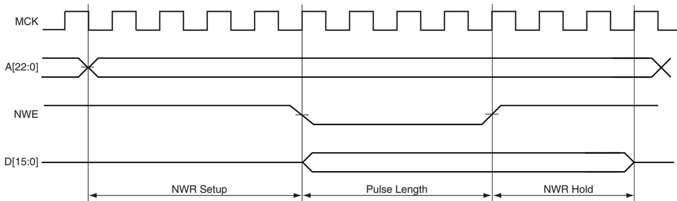
Figure 18-22. Write Access with Setup
