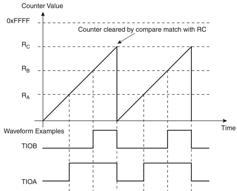
**Figure 32-9. WAVSEL = 10 With Trigger**
