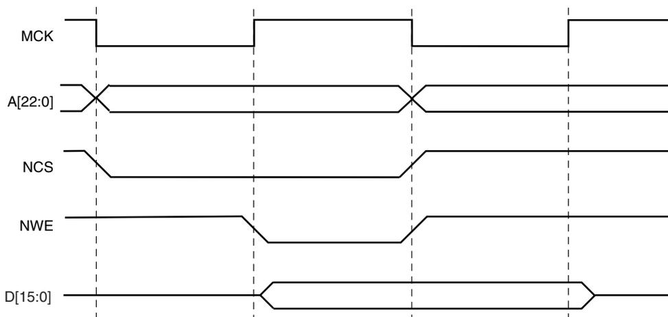
**Figure 18-10.** Write Access with 1 Wait State
