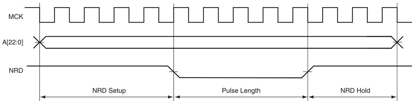
**Figure 18-20.** Read Access with Setup
