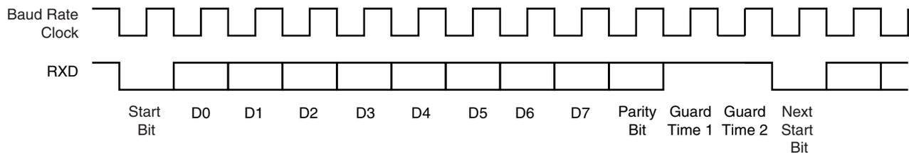
**Figure 30-21.**  $T = 0$  Protocol with Parity Error
