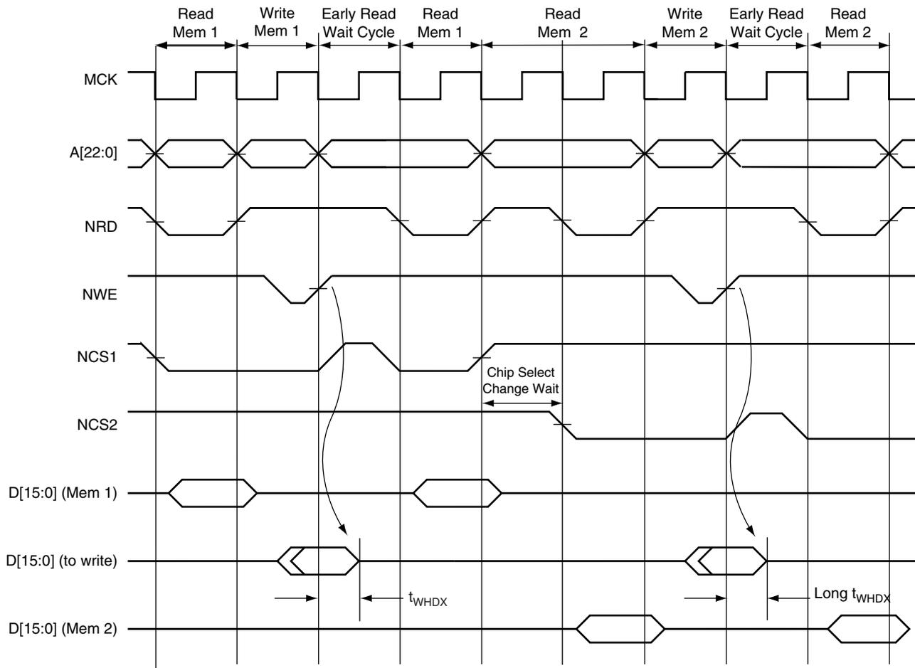
Figure 18-30. Standard Read Protocol with  $t_{DF}$
