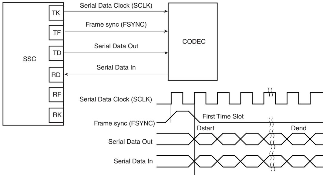
**Figure 31-18.** Time Slot Application Block Diagram
