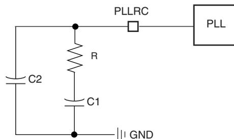
Values of R, C1 and C2 to be connected to the PLLRC pins must be calculated as a function of the PLL input frequency, the PLL output frequency and the phase margin. A trade-off has to be found between output signal overshoot and startup time.
