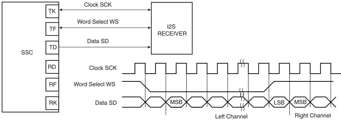
Figure 31-17. Codec Application Block Diagram
