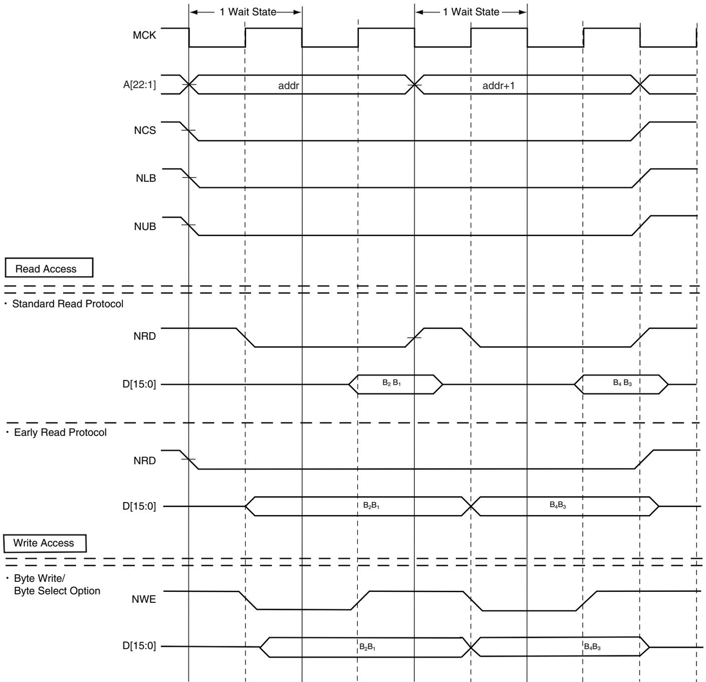
**Figure 18-40. 1 Wait State, 16-bit Bus Width, Half-Word Transfer**
