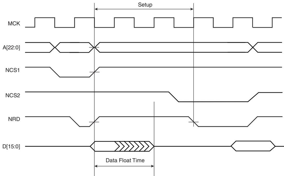
**Figure 18-25.** First Access with Data Float Wait States (TDF = 2) and Second Access with Setup (NRDSETUP = 3)
