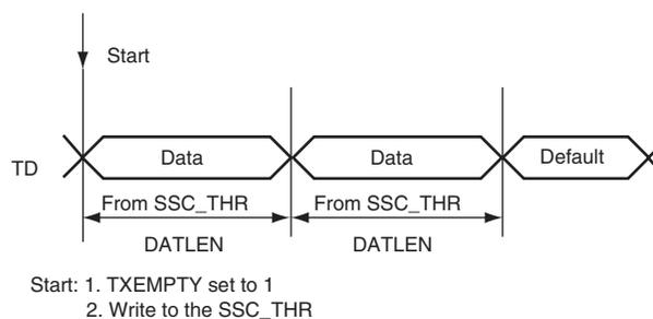
Note: 1. STTDLY is set to 0. In this example, SSC\_THR is loaded twice. The value of FSDEN has no effect on transmission. SyncData cannot be output in continuous mode.
