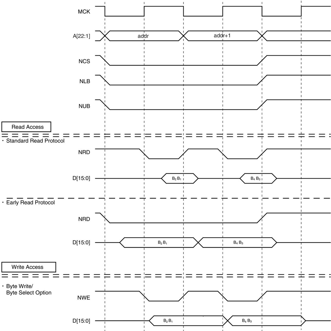
Figure 18-39. 1 Wait State, 16-bit Bus Width, Word Transfer
