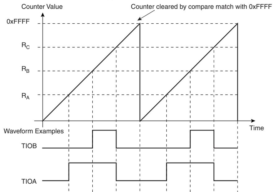
**Figure 32-7.** WAVSEL= 00 with trigger
