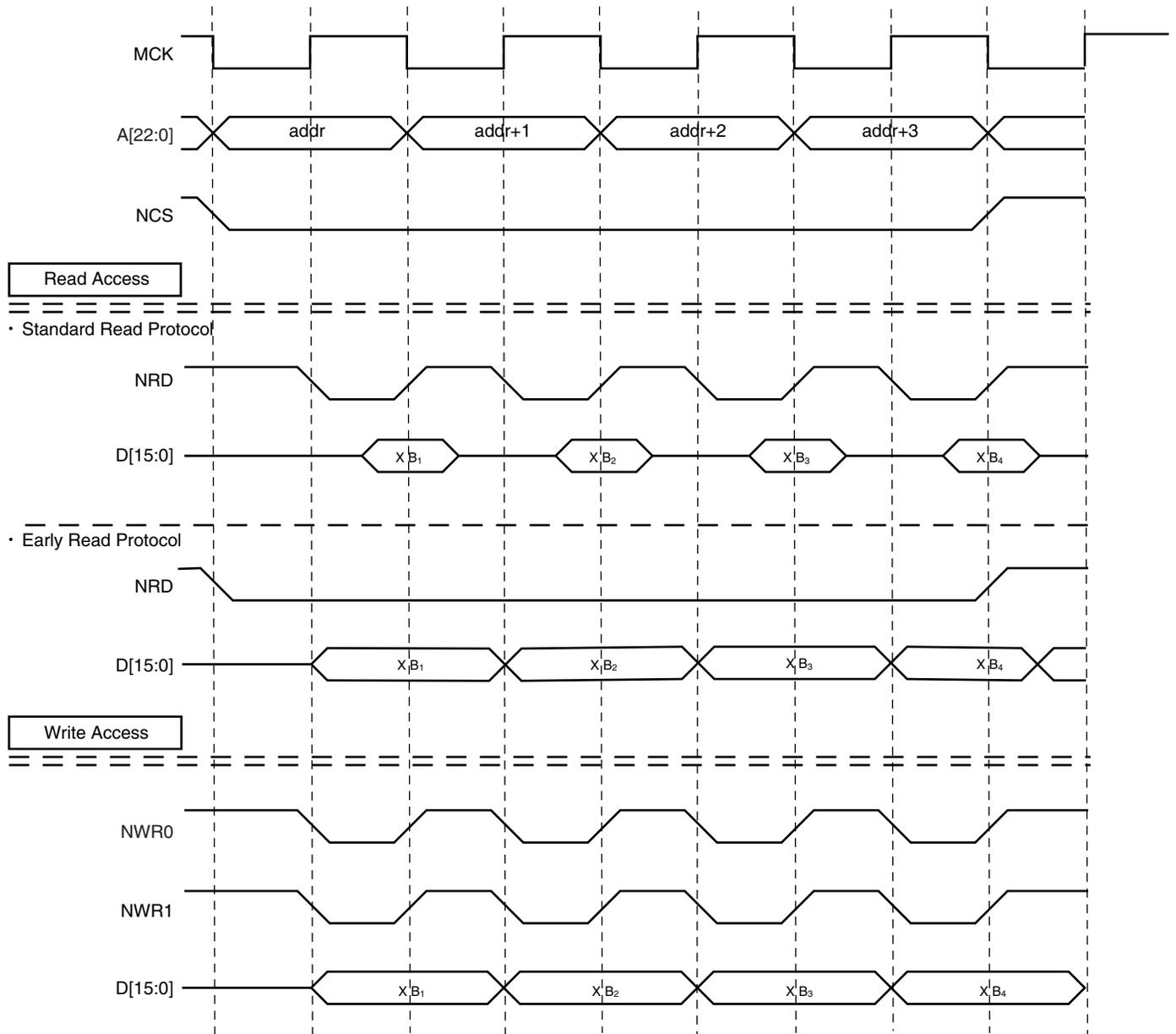
**Figure 18-42. 1 Wait State, 8-bit Bus Width, Half-Word Transfer**
