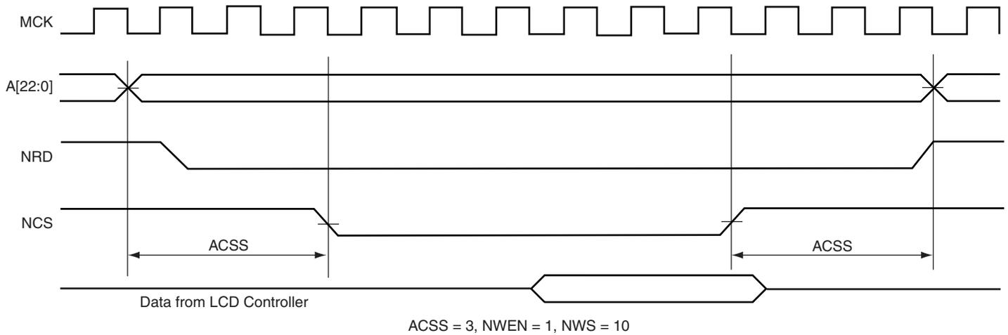
**Figure 18-27. Write Access in LCD Interface Mode**
