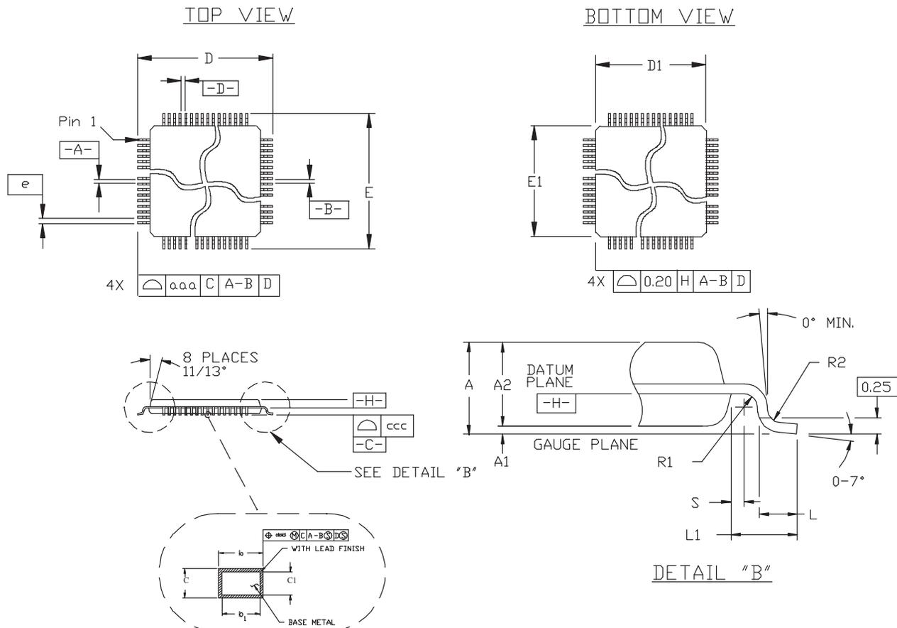
**Table 39-3.** 208-pin PQFP Package Dimensions (in mm)
