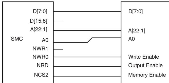
Figure 18-5 shows how to connect a 512K x 16-bit memory on NCS2 (DBW = 01).
