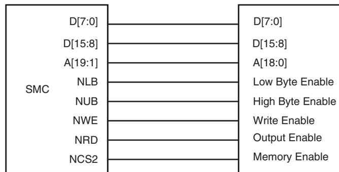
Figure 18-8 shows how to connect a 16-bit device without byte access (e.g., Flash device type) on NCS2 (BAT = 1).
