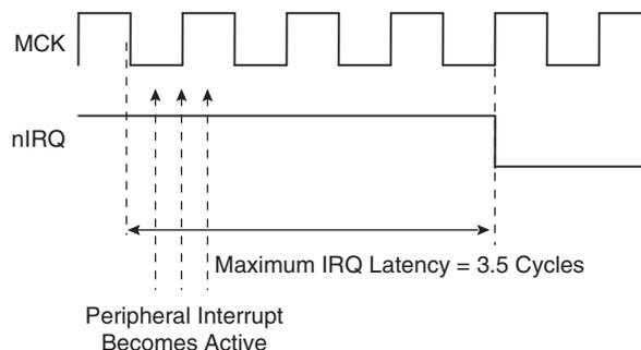
22.7.1.6 External Interrupt Source Input Stage
