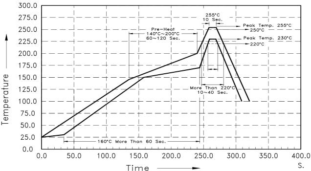
The Profile is available that must to use SnAg  $_{(x=3.3\sim3.8)}$  Cu  $_{(y=0.2\sim0.7)}$  solder paste
