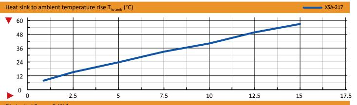
Dissipated Power Pd(W)
