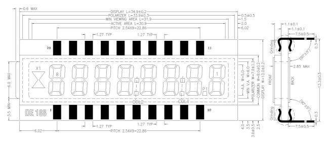
UNLESS OTHERWISE SPECIFIED DIMENSIONS ARE IN MM TOLERANCES:±0.2MM
