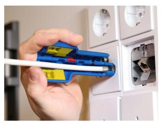
Working with WEICON Stripping tools is only permitted with potential free wires and conductions
