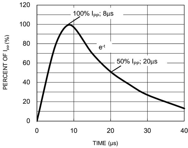
**Fig.7 ESD pulse waveform per IEC61000-4-2**
