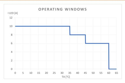
Below are the maximum current values that can be supplied by the MINI-1CV-DALI device when the working temperature varies. Ambient temperature [Ta]:
