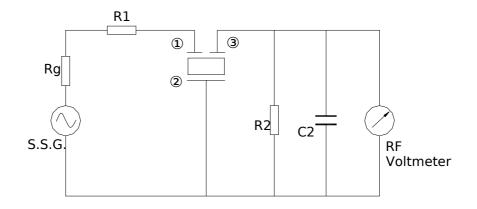
$R1=280\Omega\pm5\%$ ,  $R2=330\Omega\pm5\%$ ,  $Rg=50\Omega$ :Input
