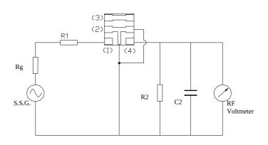
C2=10pF(Including stray capacitance and capacitance of RF Voltmeter) S.S.G: Output Voltmeter :Input :Ground :Float :Output Product Specification AEC Electronics Company Limited
