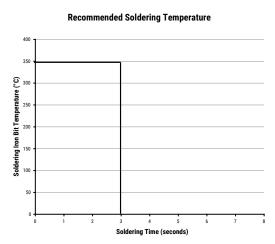
Soldering iron tip temperature should be set at 350°C (+10°C maximum), with the soldering duration not to exceed more than 3 seconds.
