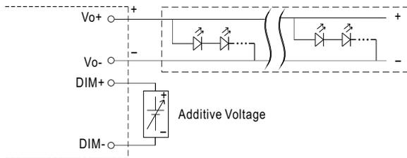
“DO NOT connect "DIM- to -V"”
