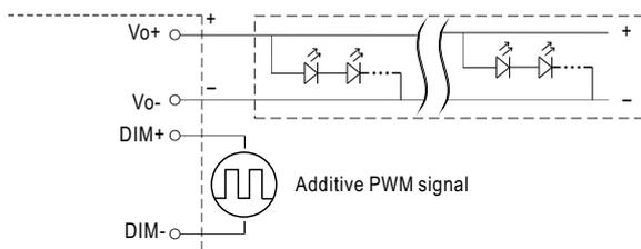
“DO NOT connect "DIM- to -V"”
