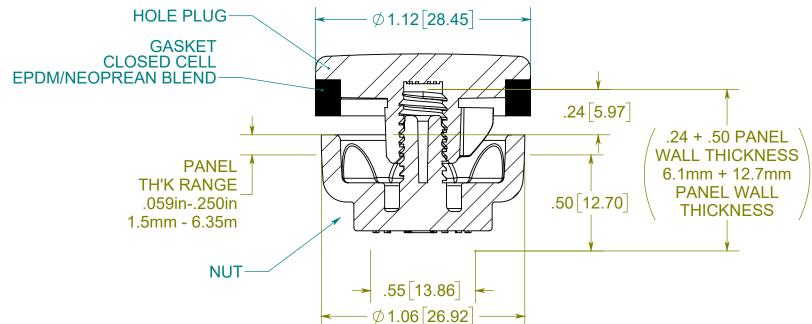
PLUGGED HOLE DIA RANGE: .625in-.812in 15.875mm-20.62mm
