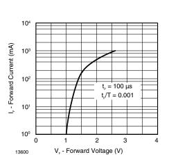
Figure 4. Forward Current vs. Forward Voltage
