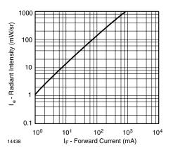
Figure 6. Radiant Intensity vs. Forward Current
