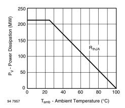
Figure 1. Power Dissipation vs. Ambient Temperature
