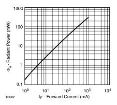
Figure 7. Radiant Power vs. Forward Current
