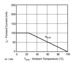
Figure 2. Forward Current vs. Ambient Temperature
