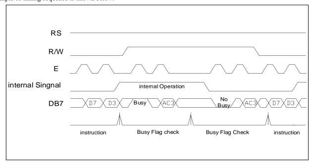
Example of 4-bit bus mode timing diagram
