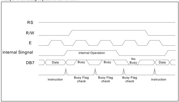
Example of 8-bit bus mode timing diagram
