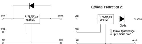
Application example: Driving a high capacitive load
